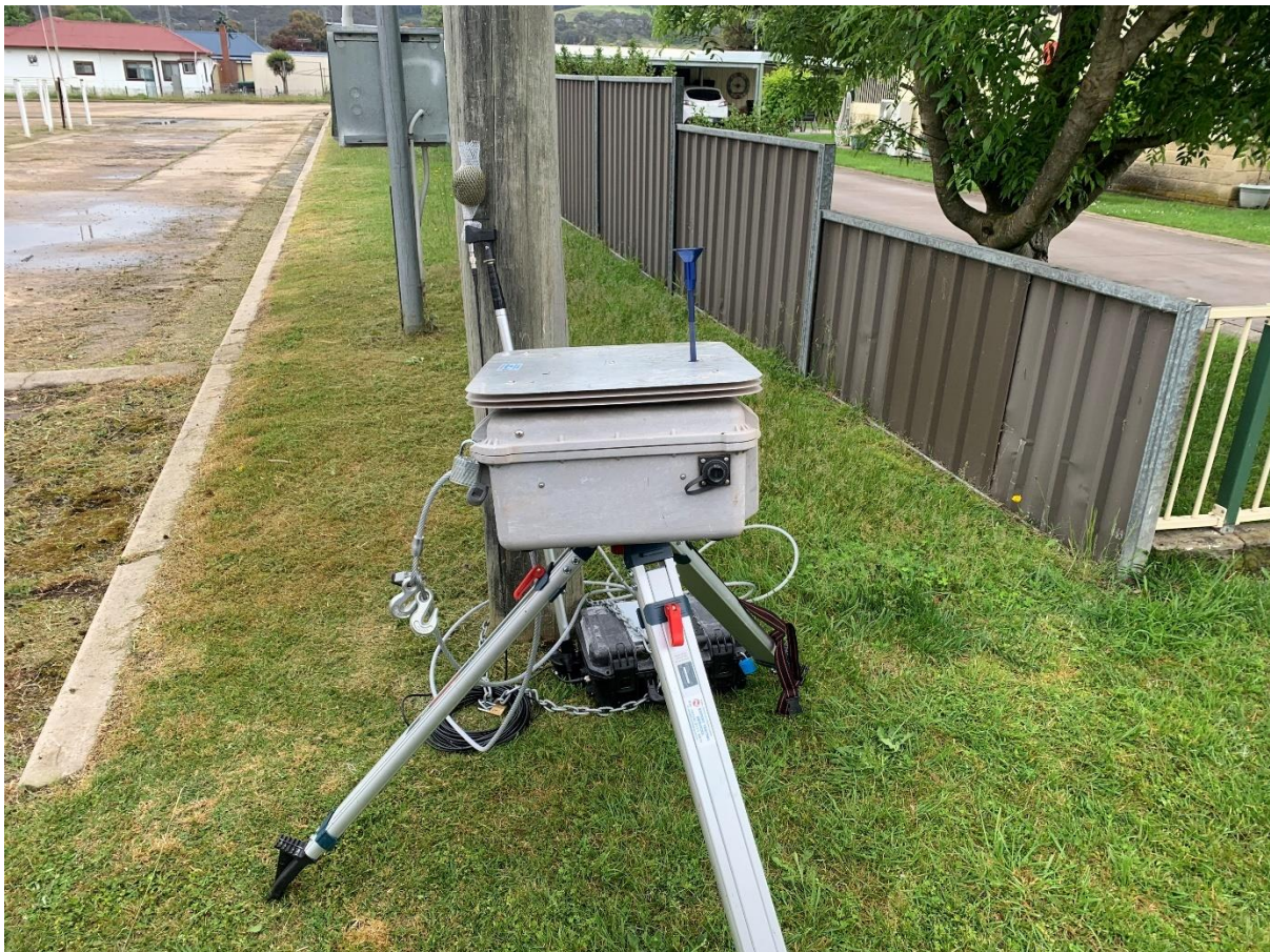
Photo 1 Depicts dust monitoring in progress
